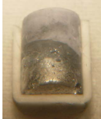
Liquid Cd cathode in Al 2 O 3 crucible
