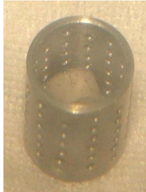
(U,Pu)N pellet in Mo crucible
