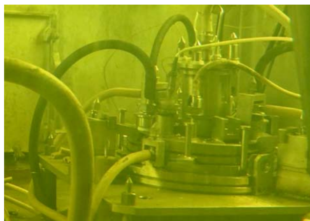
Figure 3.29. Laboratory pilot apparatus to purify salts from fission products using the sorption technique
