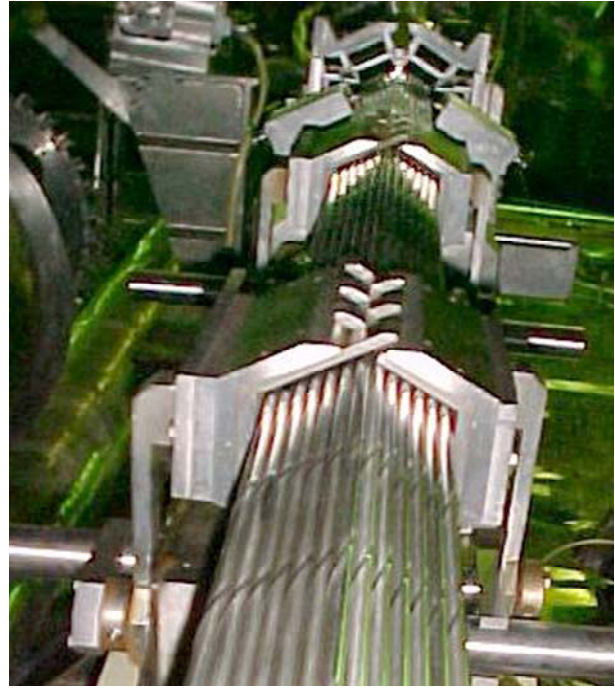
Figure 3.34. Fuel pin bundle assembling
