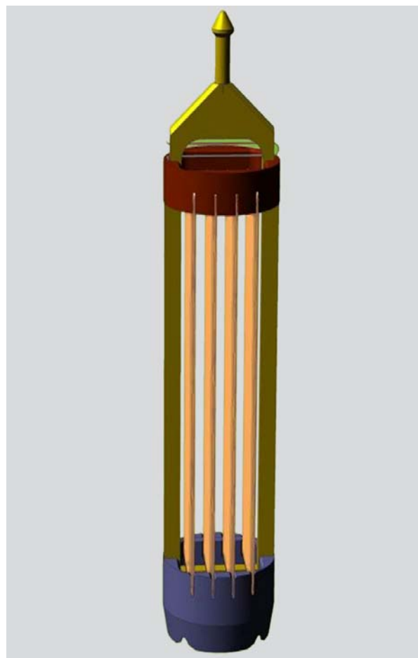
Figure 3.18. Irradiation device for 99 Mo reactor accumulation in a reactor
