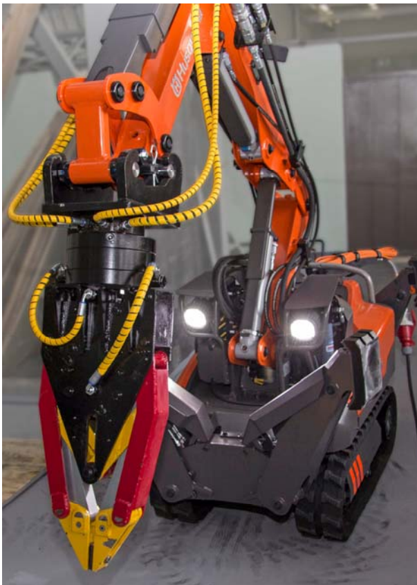
Figure 3.11. Electro hydraulic machine to perform work in the shielded box with no man present
