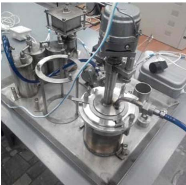
Figure 3.16. Thermal destruction facility (a) and targets welding facility (b) at the working area to produce targets accumulating trans-plutonium elements
